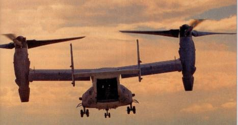
stick pressure is relaxed and the CV-22 levitates. If liftoff occurs prematurely, the Osprey will wallow and stagger a little because the wing is not yet developing enough lift to assist significantly with the takeoff. Also, the conventional flight controls are somewhat mushy, not yet fully effective. After gaining altitude following a STO, the pilot reverts to the departure profile used following a vertical takeoff.
